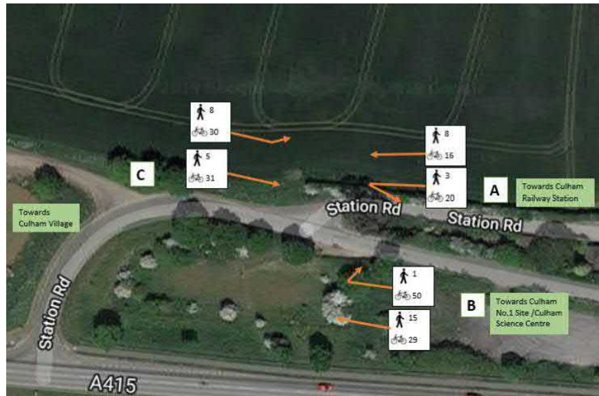
Figure 25 RIV-01: Culham Railway Station Entrance – Total NMUs observed (7-day survey period)
